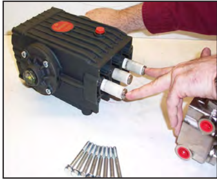
Figure 5-16. Re-install Manifold and Torque Fasteners
