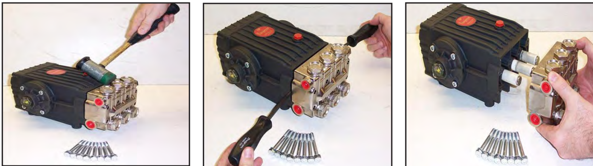
Figure 5-6. Separate Manifold from Crankcase
